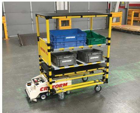
Caption CRE-553: The Creform Tite-Space BST AGV is an efficient and cost-effective material handling solution for installations with tight turns and narrow aisles.
