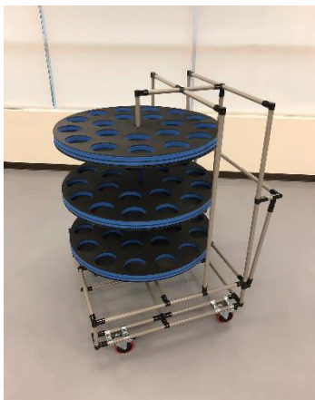
Caption CRE-596: Creform designed and built batch cart with three-level ‘Lazy Susan’ access for ease of production.
