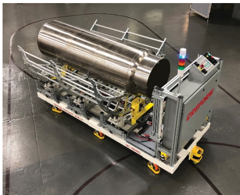
Caption CRE-604: Creform designed and built this AGV to handle large cylinders.
