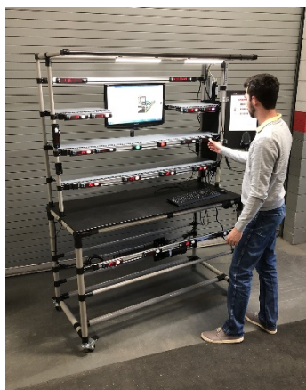
CRE-612: Creform workstation with light-guided picking.
