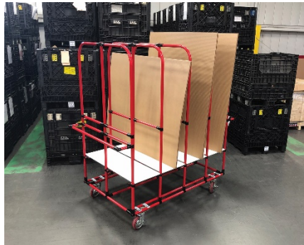
Caption CRE-618: Creform designed and built kitting cart for in-process order fulfillment.
