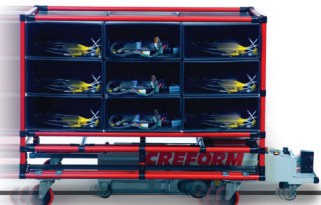
A single BST AGV can manage an entire fleet of sequenced parts carts.
