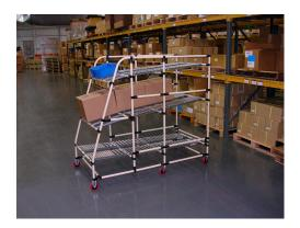
CRE-237 Caption; This mobile Creform flow rack offers pleasing aesthetics while reducing the required number of metal joints to assemble it.
