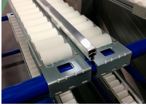
CRE-288A Caption: Aluminum, heavy duty extruded lane dividers are held by mounts secured to the conveyor rails.
