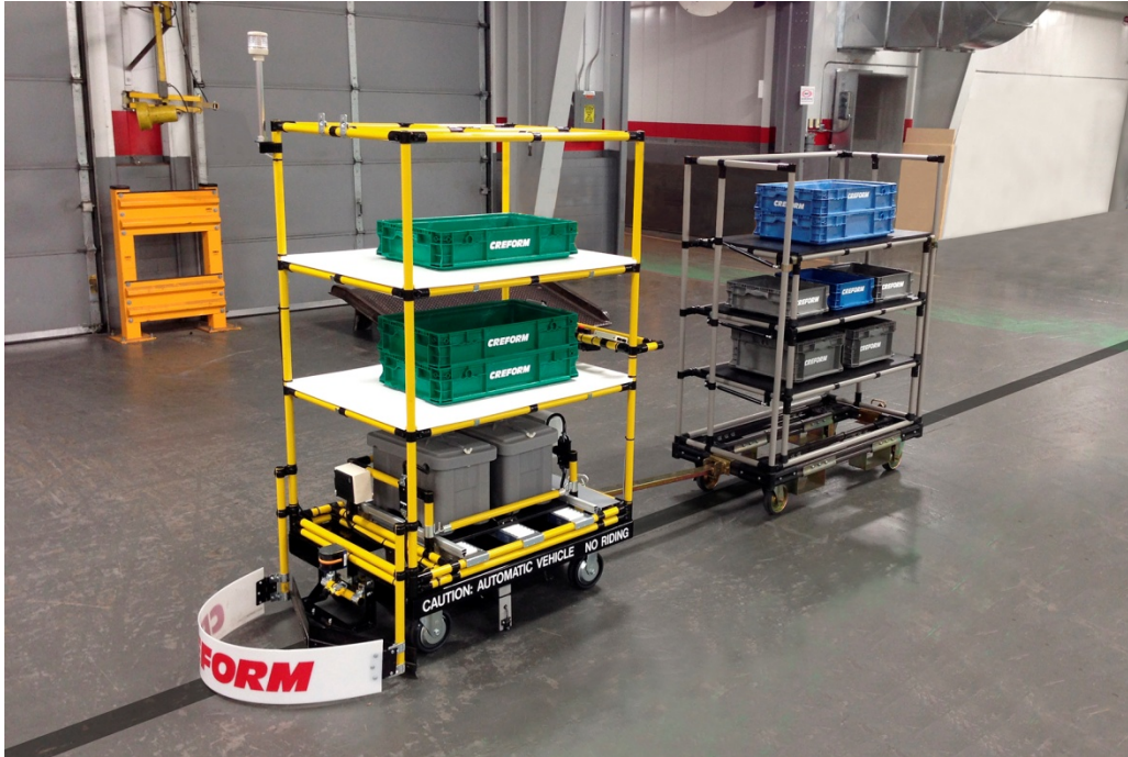
Caption CRE-537: Creform AGV Tugger with shelves pulling cart for added capacity and flexibility.
