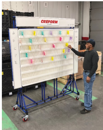
Caption CRE-624: Creform designed and built Kanban Station.
