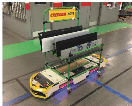
CRE-628 caption: Creform AGV Model CA-B50100-BST NSI with kitting cart.
