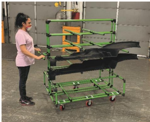
Caption CRE-635: Creform designed and built cantilevered peg cart.
