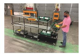
Caption CRE-643: Creform mobile flow rack features Placon® roller conveyor and a hinged section for an enhanced access.
