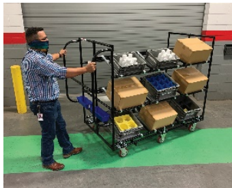
Caption CRE-645: Creform warehouse picking cart features three angled shelves on each side for the handling of totes and boxes.
