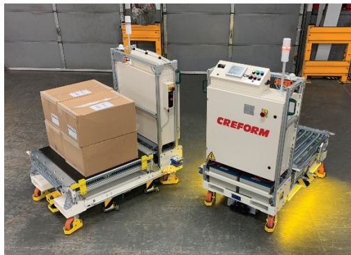
Caption CRE-650: Creform AGV with single conveyor deck.
