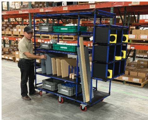
Caption CRE-653: Creform kitting cart to handle small batches.
