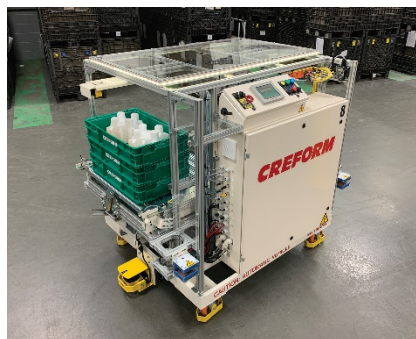
Caption CRE-654: Creform AGV with single conveyor deck.
