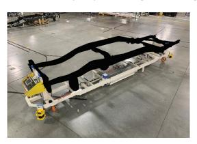
CRE-667: Creform CA-B50100-NSI, Bi-directional AGV...an unusually long AGV used to transport light truck frames. *Due to confidentiality the frame shown represents a likeness of the actual frame.*
