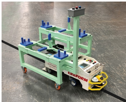
Caption CRE-669: Creform Model No. CA-250060-NSI-K9 AGV with fabricated cart.
