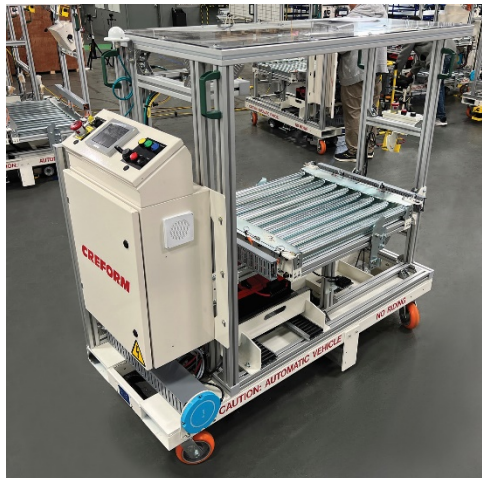
CRE-691 Caption: Single-direction AGV with conveyor deck from Creform.
