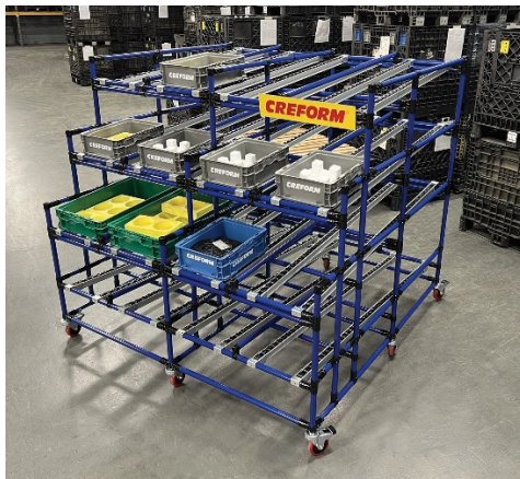
CRE-703 Caption: Creform stair-stepped flow rack for lineside presentation of parts.
