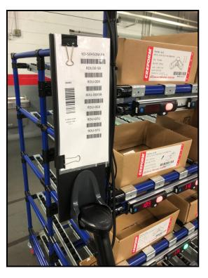
Picker runs system from barcode station. Each barcode corresponds to a recipe to be picked. Barcodes can be on a posted placard like above or on manufacturing paperwork such as traveler or work order.
