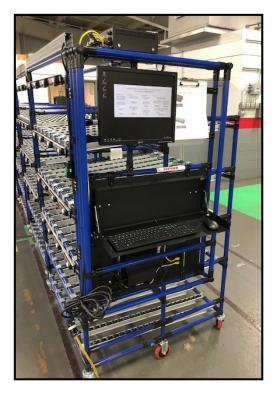
Control station positioned at end of flow rack features PC, Monitor, Keyboard/ Mouse and P2L Controller. Used for set up and general administrative support. Customer supplied PC & Monitor.
